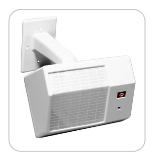
The DS794Z is a Long Range Passive Infrared Intrusion Detector which uses Motion Analyzer II Signal Processing to reduce false alarms. Several unique test features, including Motion Monitor, provide coverage integrity. Field replaceable mirrored optics, and 3 different coverage patterns provide installation flexibility.
