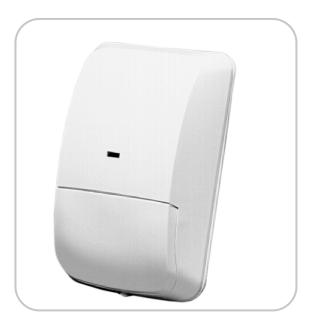
The DS303E is a wall mount, Passive Infrared Intrusion Detector which uses Motion Analyzer II signal processing to reduce false alarms. Field replaceable pointable mirrored optics, 4 different coverage patterns and 3 different mounting options provide installation flexibility.
