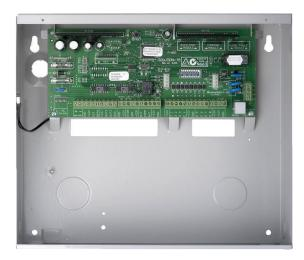
The CC880 Solution 16 Control Panel is part of an electronic surveillance system suitable for home or business needs. The control panel supports 16 zones. Eight zones use programmable end-of-line (EOL) resistor values. Add an eight-zone expansion board or use zone doubling to achieve 16 zones.
