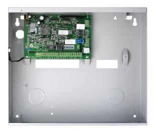
The CC488 Solution Ultima 880 Control Panel provides eight programmable hard-wired or wireless burglary zones. Remote programming provides added convenience and adaptability.
