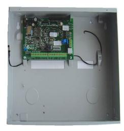
The CC408 Solution 880 Control Panel provides eight programmable zones.
