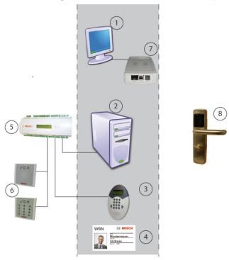
The OLS uses some components of the Online System. In the picture above the part with the grey background shows the devices which are used for both systems. On the left hand side there are devices of the Online-System and on the right devices of the OLS.
