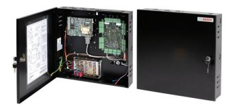
Access Easy Controller 2.1, (AEC2.1) is a new generation IP web based access controller that uniquely combines the features of a web server, video integration and security system in one complete unit. The new user interface allows more intuitive operation and improved reports capability to give the operator more control and efficiency.
