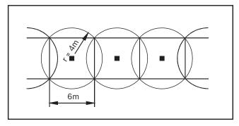
To facilitate planning for large surfaces, convert the circular detection zone into a square:
