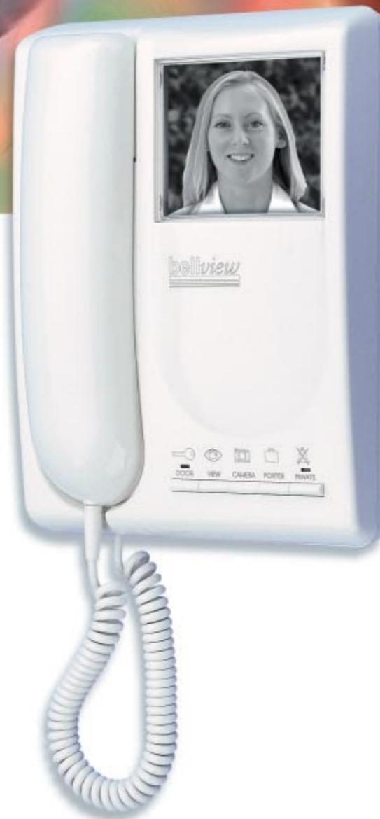
The telephone offers privacy of speech whereby only the resident who has been called can converse with the caller. When called the telephone activates the display and enables speech for a fixed period (adjustable 30 - 120 seconds). An option is available whereby the lock release button will only release the door when the telephone has been called.
