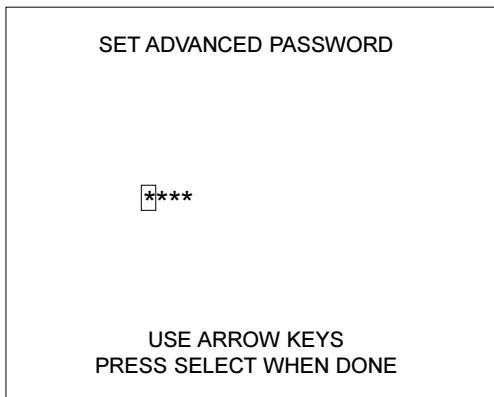
Note that the first digit of the password is selected. To change the password, the up/down arrow keys or joystick are used to select the required number for each of the four digits in the password. An up/down movement of the arrow keys or joystick will cause the selected digit to either increment or decrement. When the digit is correct, use the left/right arrow keys or joystick to move to the next digit of the password. When all four numbers have been set, press the select key.
