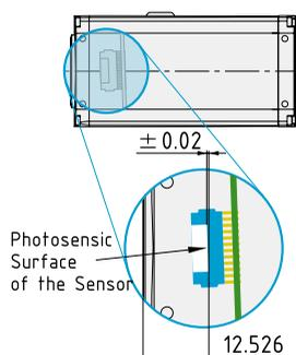
The back focal length on each camera is carefully measured and adjusted by our unique "CSAT" procedure. This guarantees an optimum distance between the lens flange and the sensor and ensures outstanding image quality based on compliance with optics standards.
