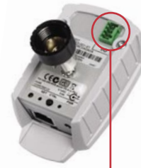
The four-pin terminal connector provides the interface to 1 alarm input, 1 output, alternative power connection. It can be used for connecting e.g. an external alarm device for triggering an alarm notification via email.
