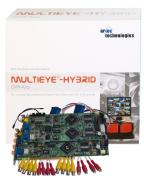
With MULTIEYE®-HYBRID DVR kits, highly professional real-time digital video recorders can be created. MULTIEYE® software supports the simultaneous operation of both analog and digital camera technologies with recording rates up to 800 ips. Up to 32 analog and IP cameras can be combined and operated with each other in one recorder as desired. Yet the integration of IP cameras is just as simple as setting up analog cameras.
