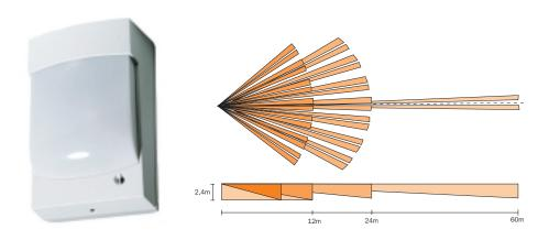
The EV 635 series provides a combined mirror optic with 24m Volumetric, 12m Volumetric and 60m L.R. detection patterns. Using a microprocessor with "4D" processing ensures maximum detection and stability. "Double Check" and "Eye to Eye" features in the EV 640 allow communication between detectors to verify alarms and minimise false alarms. EV 635 – 24m Vol./60m L.R., NC relay
