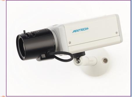
Using Ex-view HAD CCD sensor technology, the sensitivity of these models is excellent, around 0.005 lux, with low noise.
