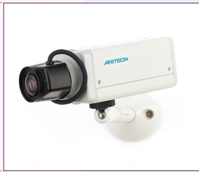
The <sup>1</sup>/<sub>2</sub>" Ex-view HAD CCD sensor is at the heart of this ultra sensitive monochrome camera. With low smear (a characteristic of this type of CCD sensor), this camera has 2 times greater sensitivity on visible light and up to 4.5 times greater sensitivity on near IR illumination (800 to 1100 mm) than conventional models.
