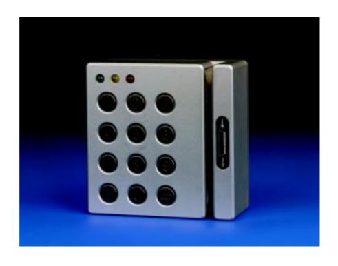
The reader can be mounted beside the doors to be controlled. Anyone requesting access must swipe a wiegand card through the slot on the reader. The reader is connected to an Aritech controller which contains the electronics to release the door. The reader is equipped with a keypad.
