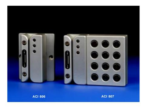
The reader can be mounted beside the door to be controlled. Anyone requesting access must swipe a barcoded card through the slot on the reader. The reader is connected to an Aritech controller which contains the electronics to release the door. The reader can also be equipped with a keypad.
