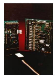
This ATD-16 transceiver unit requires no external power. The 2 wire connection facilitates easy upgrade of existing conventional circuits, leaving the wiring in place, replacing the end-of-line terminator with the ATD-16, and adding the APD-16. The ATD-16 is housed in a sealed and potted unit, takes up very little space and can be mounted adjacent to or inside of the alarm initiating device.
