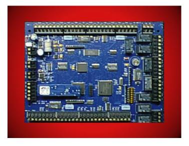
(proximity, biometrics, bar code, infrared, long range infrared), with the capability of having different readers at each port and <u>up to 4 different facility or site codes per reader</u>. It operates from +12 to 24 VDC. Quick disconnect connectors provide easy installation.
