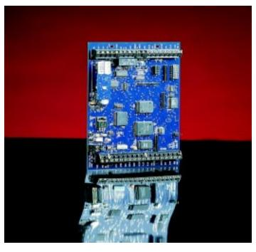
The AIM-1SL also has terminations for the door contact input, exit pushbutton, and one or two auxiliary (general purpose) alarm inputs. These inputs are all Grade "A" supervised for increased security. The supervision may be disabled when not required via a dip-switch.
