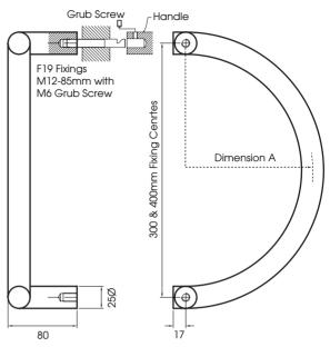
Dimension A 400mm C/C = ??mm curve 300mm C/C = ??mm curve
