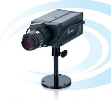
light source in that location is stable or not. Put the POE-5010HD into an IP66 enclosure with additional IR LED, it can also be used in outdoor environment. Moreover, the POE-5010HD also supports SD/SDHC slot for additiona local storage; the DI/DO plug for integrating with external sensor and alarm.
